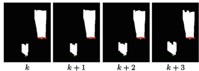
**Fig. 18** New object management. At time  $k$ , a new blob appears in the image, which already contains one existing vehicle. The new blob fulfills both spatial and temporal coherence criteria at times  $k + 1$ ,  $k + 2$  and  $k + 3$ ; thus, it is classified as a vehicle and tracked henceforth
