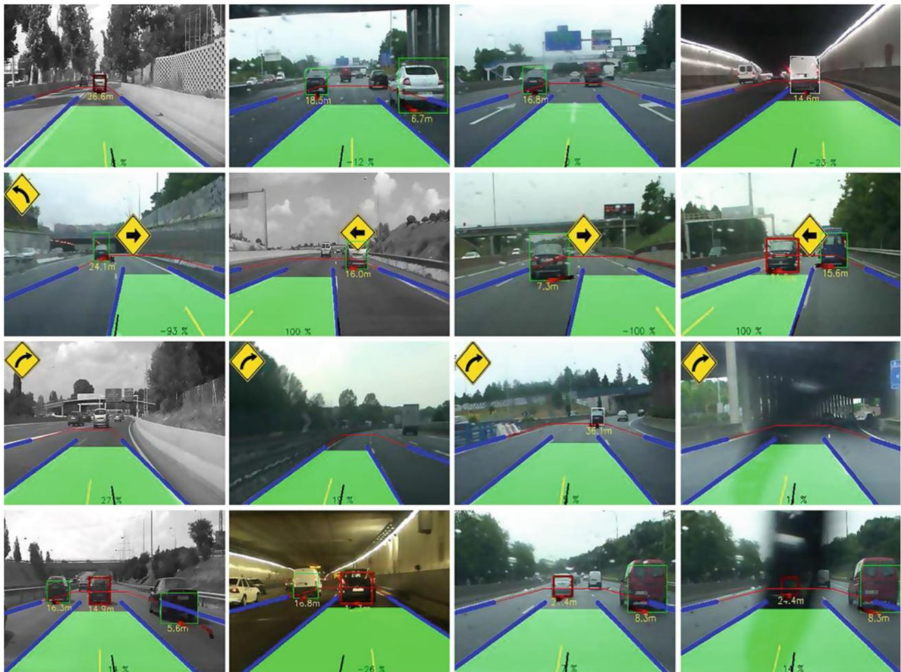
**Fig. 20** Examples showing the detected elements of the road: In the *upper row* some representative examples of the accuracy of the lane tracker are shown; the *second row* shows examples of lane change events; and the *lower row* illustrates vehicle detected in difficult scenarios
