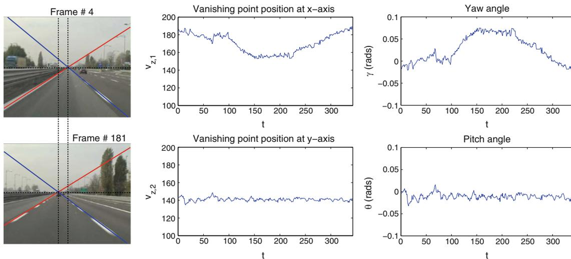
**Fig. 4** Example of variation of the pitch and yaw angle in a lane change manoeuvre. The vanishing point is shown as the intersection of *two colored lines* for a better visualization (color in online)
