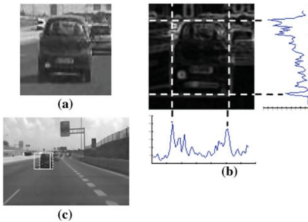
**Fig. 19** Vehicle detection refinement: **a** A detail of the closer vehicle in **c**; **b** is the result of Sobel operator over **a**. Observe that both the vertical and the horizontal edge histograms feature prominent peaks in the positions of the vehicle contour
