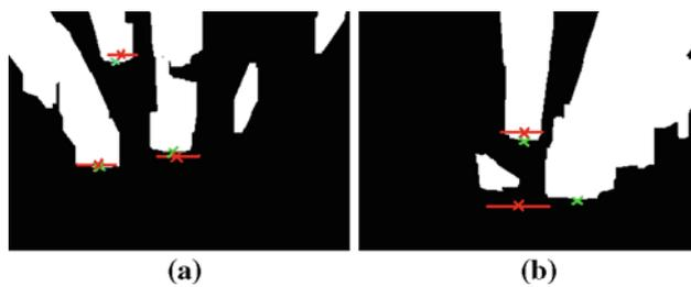
**Fig. 17** Examples of the applied clustering technique. Predicted vehicles are painted with a *solid line* and a *cross* in the middle (the *cross* indicates position  $\mathbf{x}_p$ , and the segment corresponds to width  $w_p$ ), and blobs associated with them are painted as isolated crosses
