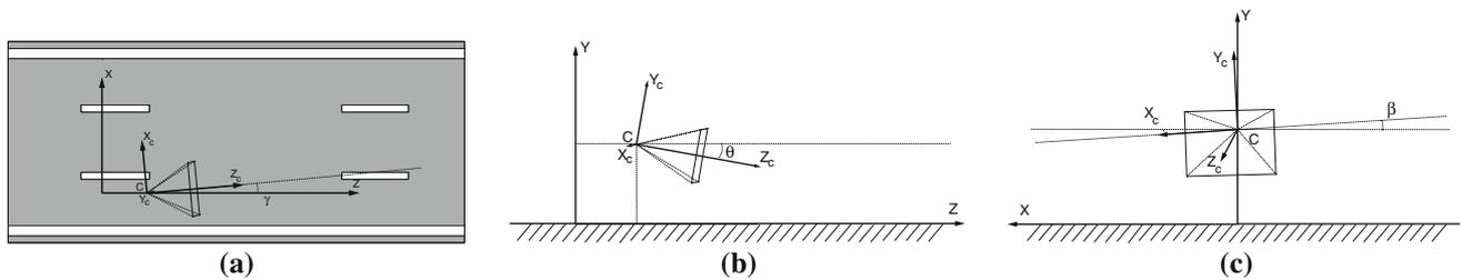
**Fig. 3** Yaw ( $\gamma$ ), pitch ( $\theta$ ) and roll ( $\beta$ ) angles, respectively in **a**, **b**, and **c** within the defined road scenario. The camera coordinate system is shown as  $\{X_c, Y_c, Z_c\}$
