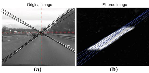
**Fig. 7** Hough transform applied to the image result of the lane marking detector: **a** least squares vanishing point depicted as the intersection of the red lines; and **b** a zoom of a lane marking for which several lines have been fitted (color in online)
