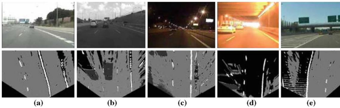
**Fig. 8** Example of the application of the Bayesian classifier to the transformed domain: *upper row* contains images corresponding to very different scenarios; and *lower* contains the segmented images. Note that the result is very accurate for all of them, except for the tunnel sequence,
