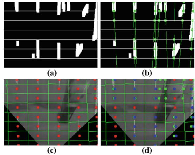
**Fig. 14** Measurement generation: **a** blobs from dilated lane marking pixels; **b** intersection of Hough lines from each blob with horizontal lines; **c** previous image with its Voronoi cells division in *solid lines*, and the set of points  $\mathbf{x}_{k-1}^i$  in *circles*; **d** current image with measured  $\mathbf{z}_k^{i,j}$ ; estimated  $\mathbf{z}_k^{i,*}$ ; and predictions  $\mathbf{x}_{k-1}^i$
