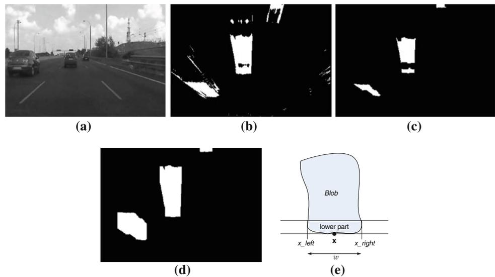
radial distortion of the elements of the objects above the road plane, as can be observed in Fig. 2. Hence, only the candidates showing a shape compliant with this kind of distortion are considered. Observe that in the example in Fig. 16d both candidates have the expected shape.
